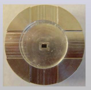
The optical flat is then mounted on a special sample holder using standard mounting wax. The die is now flat and parallel to the X-Y travel of the UltraPrep.
