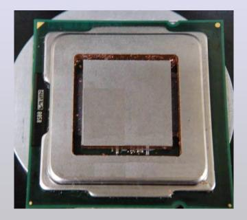
Cutting around the edges is the fastest but will not work if the heat sink is soldered to the die.
