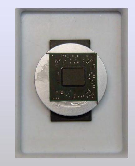
Once heated, the sample is scrubbed into the mounting wax and moved into the reference corner on the sample holder.
