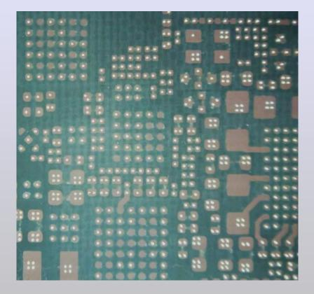
A given layer can be exposed or the entire substrate can be removed to expose components or the C4 balls of a flip chip.
