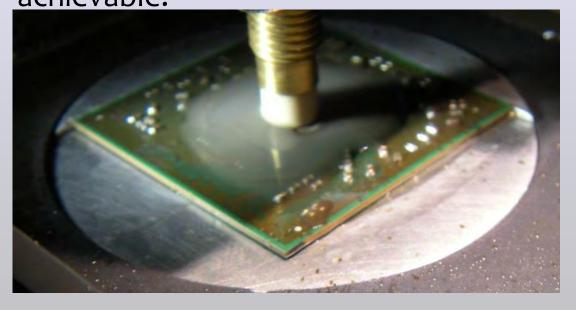
All process parameters including spindle speed, tool movement pattern, tool linear speed, and Z axis in feed are all preset. These parameters have been optimized to produce the highest quality samples.
