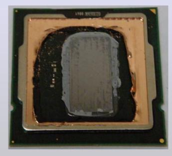
With either process, the end result is the heat sink being removed and the die exposed.
