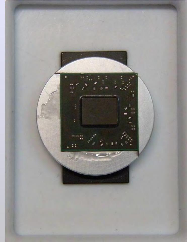
Once heated, the sample is scrubbed into the mounting wax and moved into the reference corner on the sample holder.
