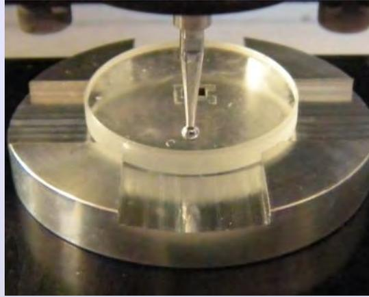
The UltraPrep will not profile the die. This could produce surface damage that results in processing artifacts. Instead, it measures the plane of the optical flat to determine the operational plane of the tool face.
