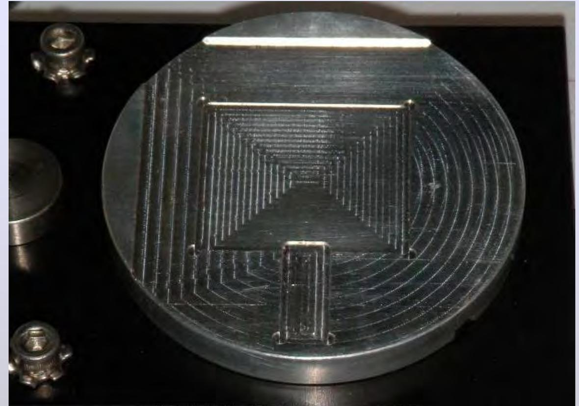
Fixtures can also be modified to align the sample center to the center of the fixture reducing die corner position movement with rotational positioning error and eliminating re-alignment between process steps.
