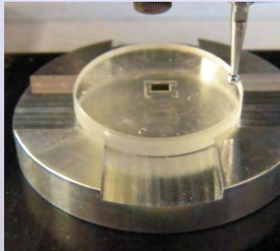
The selected lapping tool is moved in a plane parallel to the measured plane of the optical flat. If the mounting of the die was done correctly, the die surface will be absolutely parallel to the plane of the optical flat. Otherwise, the tool movement plane can be adjusted via the 'tilt' function during operation.
