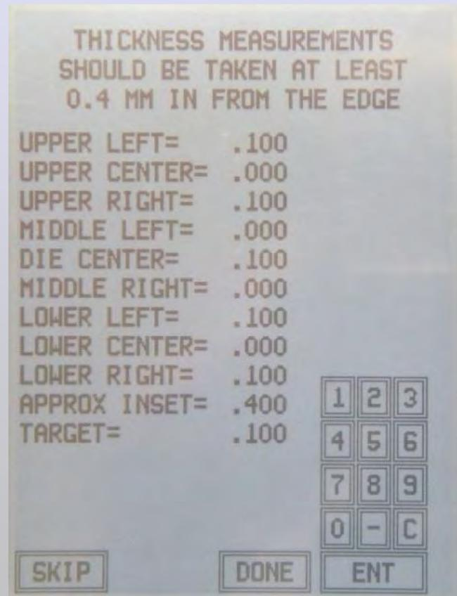
The adjustment of the profile for actual thickness measurements is required because of the redistribution of the mechanical stresses created during packaging that cause the surface curvature. As silicon is removed, the surface profile increases in curvature due to these stresses. The profile changes during silicon removal cause thickness variation as the original profile is reproduced on the processed surface.
