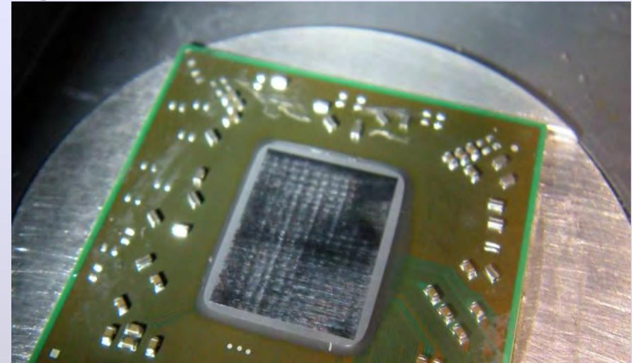
The processes are done with diamond suspension applied to the die surface. The viscosity of the suspension maintains coverage of the die surface.
