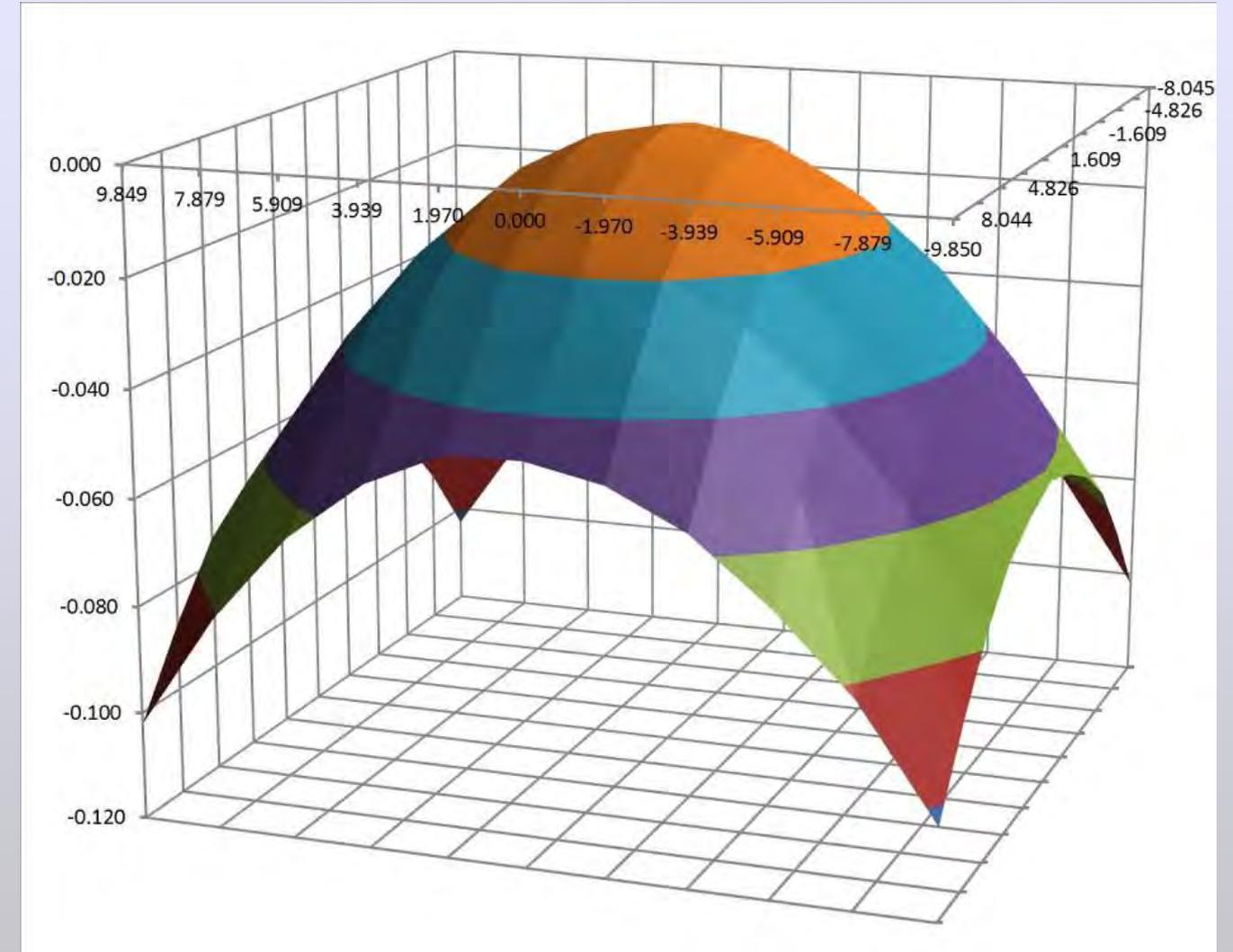
The UltraPrep measures the surface height at selected surface points creating and saving a wire frame surface representation.
