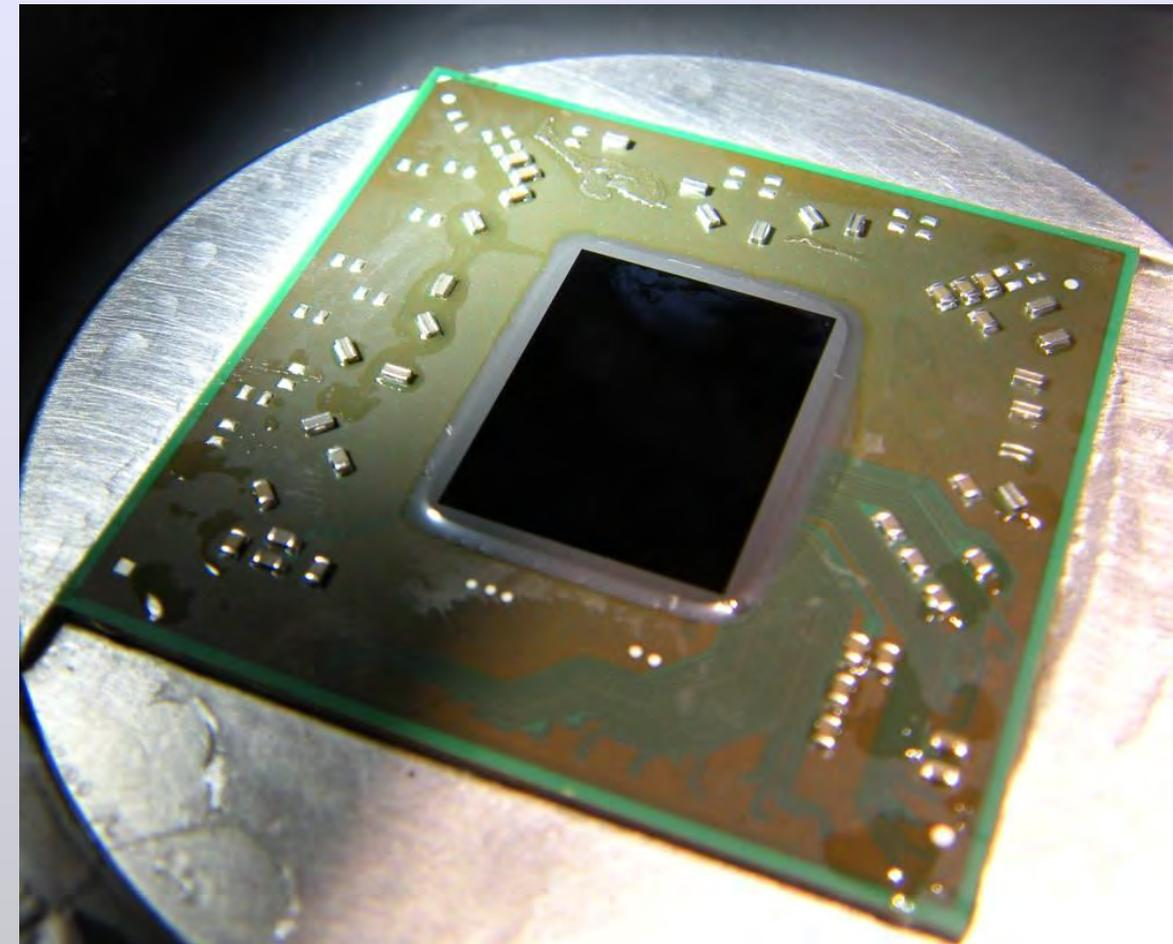
The result is a sample suitable for any additional F/A processing. The high quality surface allows easy SIL imaging and the uniform thickness speeds FIB processing.
