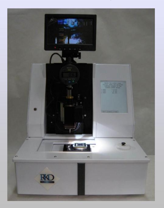
An easy to use, automatic, machining system for all mechanical sample preparation needs.
