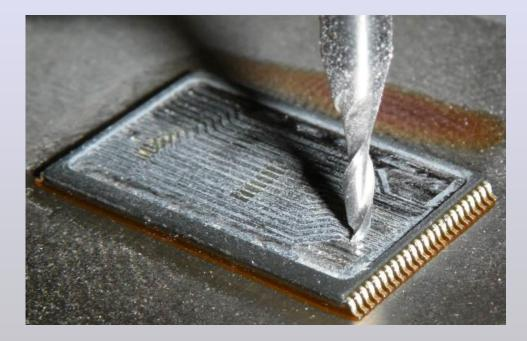
The first step is usually removing the encap and lead frame. Sometimes the lead frame can be complex and awkward to remove.
