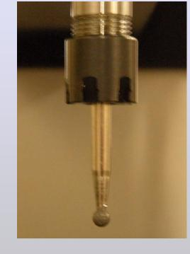
The grinding is done immersed in lubricant preventing surface heating. The forces are kept low by properly controlling tool speed, feed rate, and removal rate. This eliminates all die breakage.
