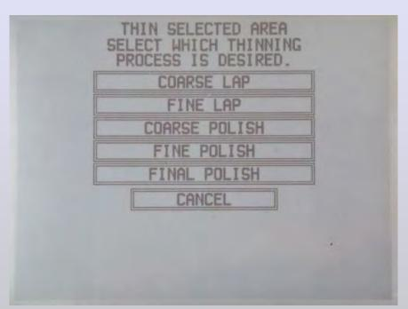
The OmegaPrep has processes available for area of interest thinning. These processes are accessed through a separate menu. The processes available and the programming of process parameters are similar to normal die thinning.
