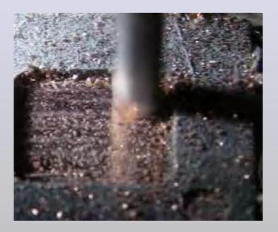
The die flag is partially removed automatically along with the encapsulant. The operator is then asked to control the tool depth so that the process can be terminated when the die attach flag is machined through. The operator then removes the remaining copper and adhesive manually.
