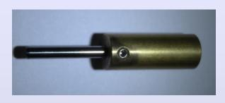
A tool setter is supplied to allow mounting tool bits properly.
