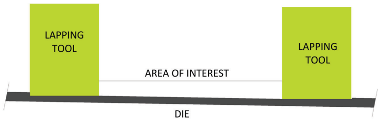
Fig. 2 As can be seen, the slope of the area of interest can be faithfully reproduced in the lower end of the cavity. At the upper end, the fillet at the cavity wall will raise the tool creating surface distortion into the area of interest.
